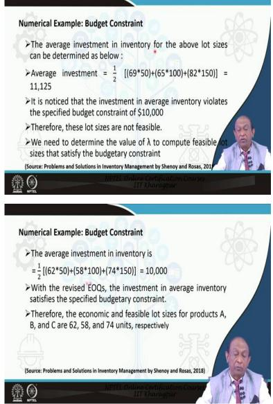
So, the average investment in inventory for this above lot sizes are the that we have determined equals Q by 2 into Cj which is 69 into 50 plus 65 into 100 plus 82 into 150 divided by 2, the Cj's are given 50, 100 and 150 and this is QA QB this is QC. So, QA by 2 is average inventory multiplied by the cost. So, this becomes 11,125.
