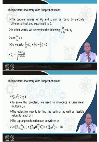
The optimal values for Qj and lambda can be found by partially differentiating this expression L with respect to Q as well as partially differentiating this expression with respect to lambda and equating both these expressions with 0. That means, del L del lambda equals 0 and del L del Qj equals 0. So, if we find out the del Qj of L equals 0 we will get this expression. So, minus Dj by Qj square into Coj plus with respect to Qj I am differentiating.
