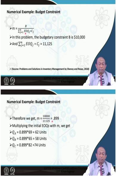
m is B by EOQ j into Cj, this particular expression in this problem the budgetary constraint is B is dollar 10,000 and this comes out to be this one. So, we get m equals 0.899. Multiplying the initial EOQs with m, we get QA QB and QC as 62, 58, and 74 units, which tallies with what we had worked out earlier, but in this case, the solution is much simpler. Thank you all.
