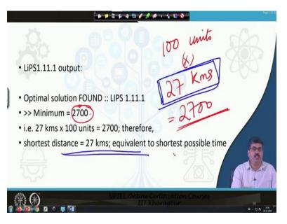
So, once we solve this, once we solve this in LiPS we get A value of 2700. We get a value of 2700. What is this 2700? 100 units multiplied by 27 kilometers is equal to 2700. So, what is the minimum distance travelled? Minimum distance traveled or minimum distance possible is 27 kilometers, agreed? So, 27 kilometers is the shortest distance from factory to my destination point.
