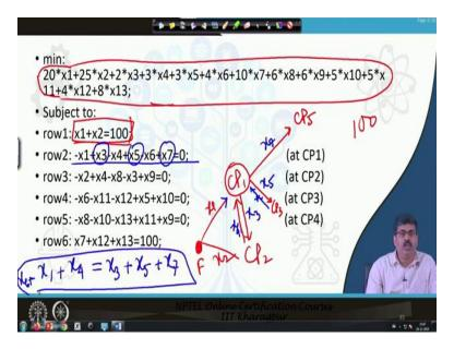
So, what is our objective? Our objective is to minimize the total distance traveled. Minimize the total distance travelled, distance traveled is 20, say the first 1, take the first 1, this 20 kilometers distance, 20 kilometers distance how much quantity is being taken, x1. 25 kilometers is the distance from 1 check post to the other, how much quantity is being taken, x2.
