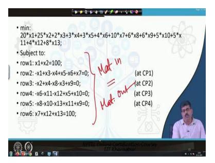
So, this is my, all these constraints are given here, all these constraints we have put equal to on the right hand side just for modelling simplicity purpose, but otherwise it is x1 plus x2 plus x3 is equal to x4 plus x5 plus x6 material in material out, material in is equal to the material out. Remember this material in is equal to material out because we will require this in the subsequent lecture sessions also.
