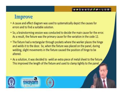
So, now, improve stage we are trying to say conduct the cause and effect analysis to depict the causes for the errors to find a suitable solution. So, a brainstorming session was conducted to decide a main cause for the error and fixture was primarily cause for the variation in the code 12. So, we add the problem with code 12 maximum number of defect we have also seen there was a problem with the measurement, we had seen that sample number 15 was indicating out of control process.
