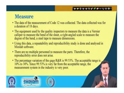
Now, in the measure phase this is the define phase what is the problem? Now in the measure phase. So, their data for the measurement of code 12 was collected and the data was for a duration of 18 days. So, the equipment used by the quality inspectors to measure the data is the Vernier caliper, we have to define all this and the band of the sheet a right angle scale to measure the degree of the band steel tap to measure the dimensions.
