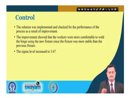
So, many things where thought as a part of critical thinking cause and effect and the appropriate action is taken to put and additional sheet to make your say welding position are quite accurate and the hinge welding stable. Finally the control phase the solution was implemented and checked for the performance of the process, as a result of improvement and the improvement showed that workers were more comfortable to weld the hinges they were having better and control.
