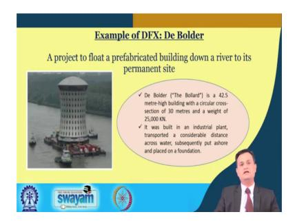
Just see the example of De Bolder you might be aware and this is a project to float a prefabricated building you see such a gigantic building down a river to its permanent site and this is a 42.5 meter high building with a circular cross section of 30 meters and a weight of 25000 kilo Newton.
