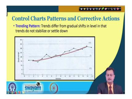
There is it trending pattern. So, some trend you can observe maybe because of wear and tear of the tool bearing or some other say component or there maybe some error in the measuring instrument.
