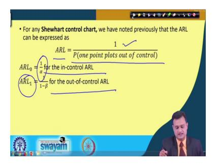
So, here your ARL is basically 1 divided by we have seen this in detail. So, ARL is 1 by probability, one point plots out of control. So, this can be given by 1 by alpha, and this is in control ARL. So, this is for in control ARL and when I say ARL 1 for the out of control 1 upon 1 minus beta.
