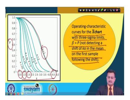
So, let us try to see the graphs that will help us. Now this is the operating characteristic curve for X bar chart, with 3 sigma limit and beta is equal to probability of not detecting is shift on the first sample, following the shift means, shift has occurred. After shift has occurred I took the sample and I am not able to detect this on the first sample after shift has occurred this is typically my beta probability of non detection type 2 error.
