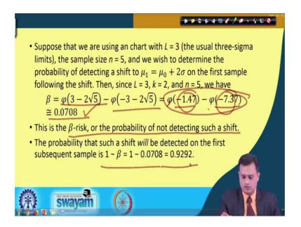
So, I will just put the values. Let us say I am taking the value. Suppose that we are using a chart with L is equal to 3, the usual 3 sigma limits, sample size is n is equal to 5; we wish to determine the probability of detecting mu 1 is equal to mu 0 plus 2 sigma. So,
