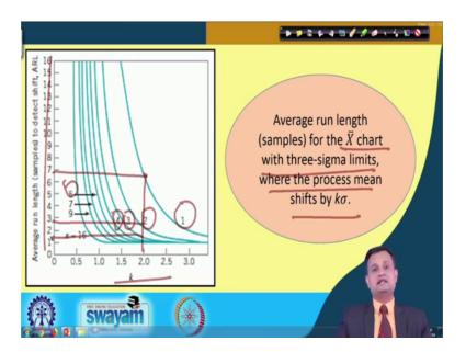
So, we have already seen this expressions in detail. Now just let us try to appreciate this in terms of the OC curve. So, or typically ARL curve here. So, average run length curve for X bar chart with 3 sigma limit by k sigma shift this remains same the logic remain
