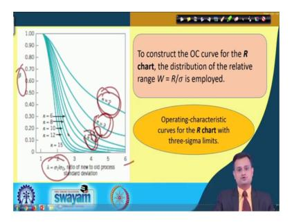
Similar way I can plot the OC co for R and here I am considering lambda is equal to sigma 1 divided by sigma 0, because for R chart I am considering that there is a shift in the variability my original variability let us say sigma 0 it has got shifted to sigma 1.
