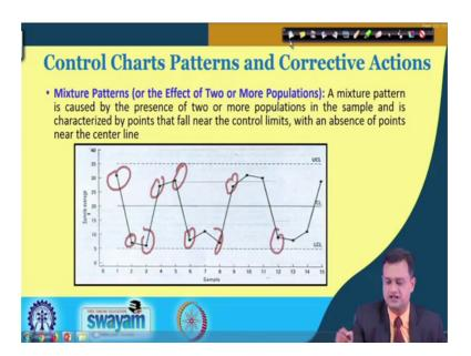
You can see another that is the mixture pattern and you see the points are falling very close to the control lines maybe upper or lower and this is typically called mixture pattern.
