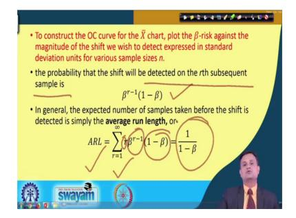
Now, once you are done this the remaining task is very simple. So, you have to construct the control chart sorry OC chart OC curve for the X bar. So, you need to plot the beta risk against the magnitude of the shift. We wish to detect in standard deviation units, for various sample size and in standard deviation unit means my mean got shifted by 2 sigma, 3 sigma, 4 sigma what?
