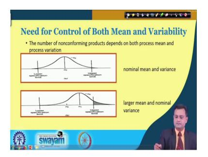
Now, let us see couple of cases to appreciate the need for control for both mean and variability. So, I am talking about the control chart for variables and I would emphasize that I must have X bar chart that used for mean and I must have R or sigma or S chart that is for variability and these two are complementary to each other. So, I will not say that only go by X bar or only go by R.
