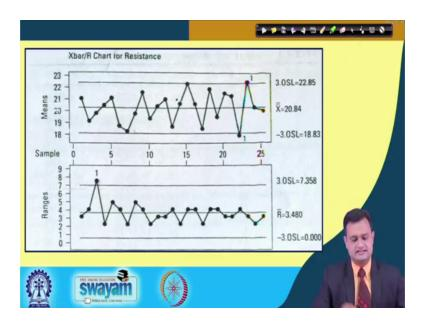
So, now once you have done this you can plot the data and data means what? You will plot the values of X i bar, it means you will plot the values of average of each particular sample and you have X double bar is a centre these are the means which is X i bar and this is X i bar and here you will plot the values of R i and this is your basically R bar.
