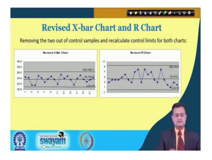
So, I will exclude this points once again I will calculate the control limits and then once I feel that my control limits are stabilized I will go for. So, this is the recalculated control limits more or less it is falling within the control limits I will accept this my gauge is ready for implementation gauge is my control chart.
