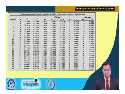
So, you find the upper control, lower control for X bar chart and S chart once this is done, then you can see this table also, that I have put all the values of X bar S you will see the value of A 2 LCL, UCL which is basically which has used the value of A 2, B 3, B 4 and the S chart.
