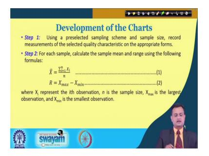
So, this is exactly what we do, so if we quickly go through the general steps for constructing a control chart then step 1 using a pre selected sampling scheme sample size, record measurements of the selected critical quality characteristic on appropriate form. Step 2 compute X bar R which is the X bar is the average of your all the measure the readings for the given quality characteristics, R bar is within sample maximum minus minimum.
