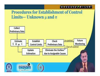
So, once you are done with this, then I have simplified everything through a simple flowchart and it goes like this collectively preliminary data then estimate X double bar R bar S bar establish control limit this will be called trial control limits. Check preliminary
