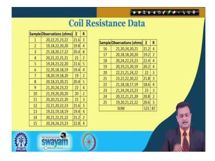
And then this is the data you have, so you have the sample 25 sample each sample has 1, 2, 3, 4 1, 2, 3, 4, 5 reading. So, your sample size is 5, you compute the X bar for each particular sample I will call it as X i bar and then R, a total is 521 that is the X bar value R is 87. So once you understand, so that I need not to explain for every example.
