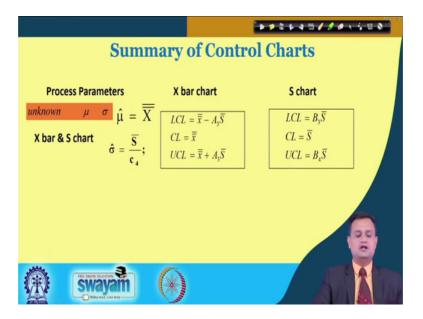
This is again for unknown mu and sigma X bar and S chart, so you can easily make use of this control limits and plot the data, set the trial control unit plot the data, get rid of the points outside the control limit make your control chart gauge perfect and then implement.
