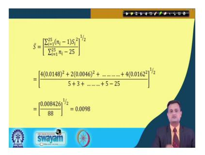
So, this is my initial computation for X bar and S chart I computed the S bar by using the expression I have given and once this is done, then for n 1 is equal to 5 X bar chart you can compute UCL as well as LCL.
