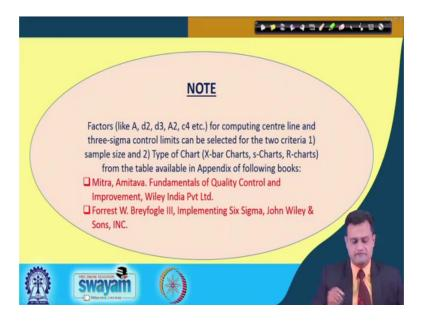
So, typically you need to refer couple of say standardise values. So, factor likes A, d2, d3, A2, c4 etcetera, for computing the central line and three sigma control limits, they can be selected from the table based on 2 criteria number 1 sample size and number 2 type of control chart X bar chart, S chart or R chart you are using.
