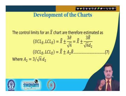
So, then you will have the upper control limit and lower control limit for X bar, so it would be X double bar plus or minus 3 sigma hat divided by square root n and you can put sigma hat is R bar by d 2 and this word give X double bar plus or minus A 2 R bar because A 2 is 3 sigma root and d 2. So, 3 sigma route n d 2 is my basically A 2 and I can just simplify the value of A 2 can also be read from the table.
