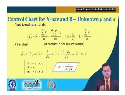
So, in this case you have to estimate mu hat X bar is equal to X double bar and you have sigma X i bar i is equal to 1 to m divided by m; m is basically samples and n is the
