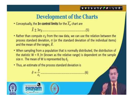
Then you compute the 3 sigma control limit X double bar which is the central line plus or minus 3 sigma X bar and sigma X sigma hat basically is R bar by d 2. So, this I can very easily find d 2 I can find from the table.
