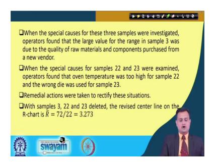
So, based on this some say conclusions were drawn that. When the special cause for sample 22 and 23 on X bar chart where examined operator found that temperature was too high for sample 22 and the wrong die was used for sample 23. So, this you have to investigate you may have to do brainstorm, you must have a process knowledge and typically remedial actions were taken.
