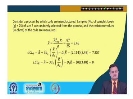
So development of X bar and R chart for coil manufacturing process, the data is like this you have a process which manufactures the coil and samples number of sample taken at 25 size 5 are randomly selected from the process and resistance value in ohm are measured. So, R bar you can compute, you have UCL R, so D 4 R bar D 4 is from table you get this LCL R this is 0 say maximum of this so by chance if it comes out to be negative then you will take 0 as I discussed.
