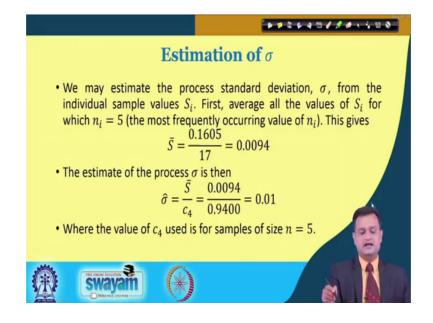
So, we have computed the upper control limit, lower control limit for X bar chart as well as S chart and I can also estimate the sigma S bar is equal to 0.1605 divided by 17. I will just consider the samples which has the sample size 5 and then I will take the submission of all the S i of this number of sample here it is 17 sample which has sample size 5. So, I will get the S bar 0.0094 and sigma hat is this for n is equal to 5.
