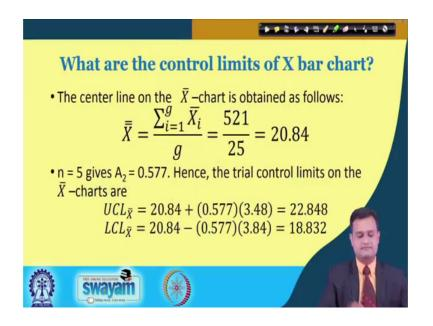
You compute the X double bar and then you compute the UCL X bar and LCL X bar. So, this A 2 is from the table for n is equal to 5 and the X bar chart. So, only two thing sample size and the kind of chart you want to plot you will get the value of the constant from the appendix of the suggested textbook standardised table.
