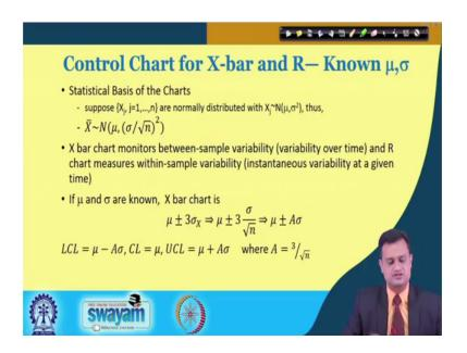
So, you have let us say X j is equal to X j is equal to 1 to n and this is normally distributed with X j n mu is the mean and sigma square is the variance and the distribution sample distribution is X bar which is also normally distributed and you can
