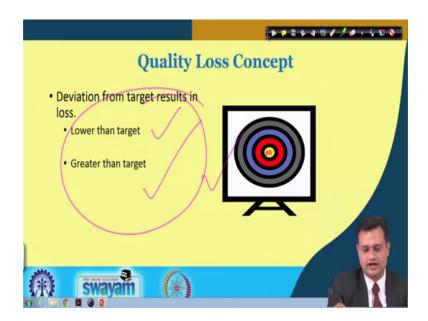
So, typically quality loss function, you can see this figure. This is my target, where I want to achieve my performance lower than target and greater than target, both are the losses. I cannot afford to have this.
