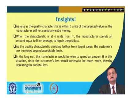
So, these are the insights as long as the quality characteristic is within delta, the targeted value of m, the manufacturer will not spend any extra money, when the characteristic is at delta unit from m, the manufacturers spans about equal to B, so that my customer does not feel unhappy to repair the product. As the quality character is deviates further from target value, customer loss increases and I must see the trade-off.
