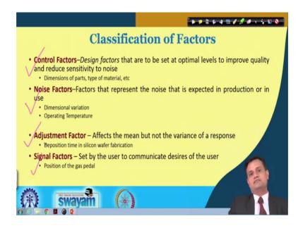
Now, there are a couple of key terminologies that I would like to define. One is the control factor, so this is typically the design factors that are to be set at optimal levels to improve the quality and reduce the sensitivity to noise. So, it may be the dimension of part type of material. There are noise factors, this particular factors, they represent the noise that is expected in production or in use some dimensional variation, operating temperature and so on.
