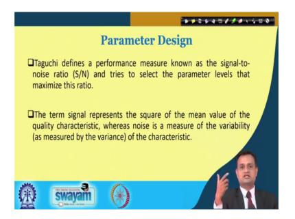
So, Taguchi concept is basically parameter design concept. And he tries to do this with the S by N ratio, signal to noise ratio. Objective is to use the orthogonal array, objective is to consider the noise factor, controllable factor, and design, and execute the experiment in such a way that S by N can be maximized.
