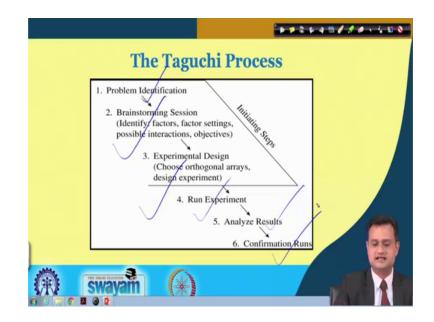
So, this is typically the steps; problem identification, brainstorming identification of factors, noise as well as control, setting objectives, experimental design based on orthogonal array, run experiment, analyze results, and confirmation of the runs.
