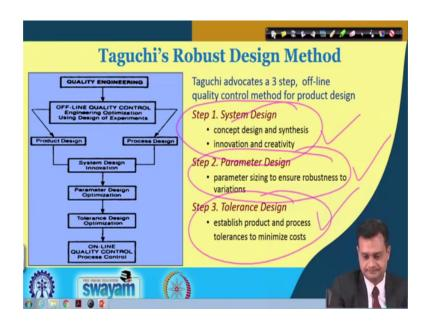
And these are the steps of my Taguchi's robust designed method. First is step-1 that is the system design concept design and synthesis, innovation and creativity. Step-2 parameter design, parameters sizing to ensure robustness to variation. And 3rd is the tolerance design, established product and process tolerances to minimize the cost. Remember this is the best stage to apply the concept of Taguchi. As you advance from here to here to here, your complexity increases.
