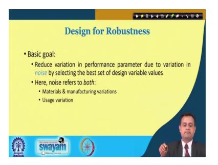
So, designed for robustness is to minimize the variation because of noise.
