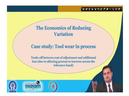
Now, let us see the economic reading variation, and there is a case study of tool wear in the process. Now, here you need to analyze the trade-off between cost of adjustment and additional loss, due to a allowing process to travels across the tolerance band. So, the situation is like this, I have a machinery. I would expect that machinery to be set at a particular value target value produces the nominal targeted dimensions.
