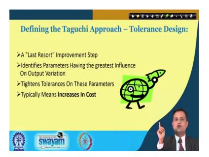
So, this is the tolerance design is the last resort. So, typically when you are going to step three, this will increase the cost, and we are trying to tighten the tolerances. Obviously, to produce those tolerances, you need to have very high end machinery equipments and precision as well as the measuring instrument, this will increase your cost, and this is not desirable. Try to focus on the system states through innovation, and then parameter straight through Taguchi design.
