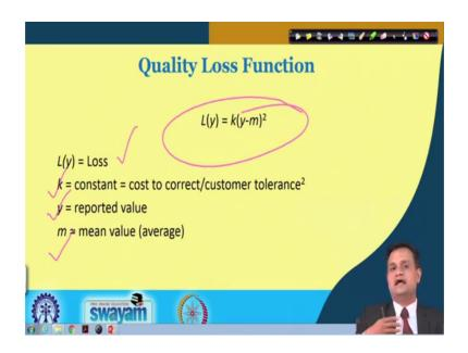
So, this is the quality loss function, Taguchi has proposed L y is equal to k y minus m whole square. So, L y is the loss function, k is the constant, y is the reported value, m is the mean average or targeted value. As you deviate from the target, my loss function is quadratic in nature, and it increases lost to society is increased. So, this is my quality loss function.
