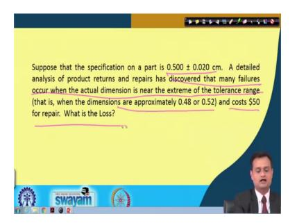
So, I have the illustrative example. Let us say you have a part 0.5 plus or minus 0.02 is the specification. And you have discovered that many failures occur, when the actual dimension is near the extreme of the tolerance range. And approximately dimensions are 0.48 to 0.50 cost is 50 dollar for repair, what is the loss.
