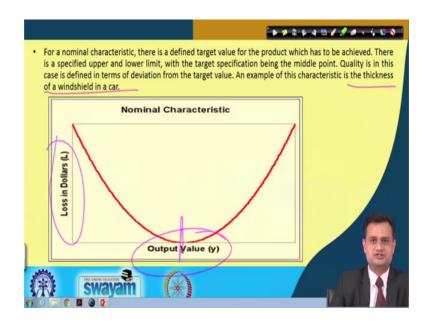
So, once you have these expressions, you can just try to analyze that what does it mean. So, when I say nominal characteristic, and typically what do you see here, this is the loss, and this is the output variable Y. So, an example of this characteristic is the thickness of a windshield in a car. And in this case, you would like to have the target value. So, here target is the best, nominal is the best, this is the example of nominal is the best.
