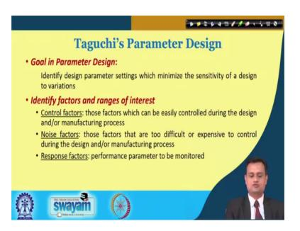
So, finally intelligence design, goal in the parameter design is to identify the factors and ranges of interest for control factors, then noise factors, and the response factor.
