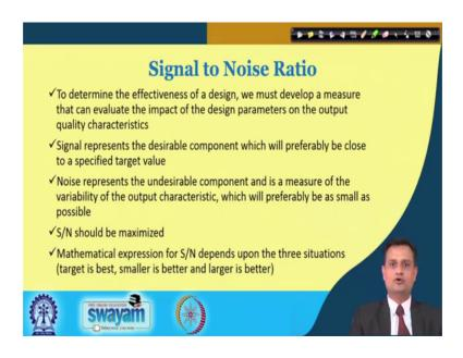
So, this example will really help you to appreciate that what is the concept signal to noise ratio, signal is something desirable, noise is not desirable we all know, and signal to noise ratio must be optimized.
