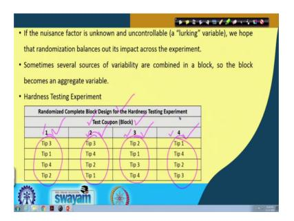
Now, just see the example here and what is the example that, you have some uncontrollable factor lurking variable also it is called and let us say I have a machine for testing the hardness of the specimens or the material and I have some test coupon. So, you can see here that randomized complete block design for the hardness testing experiment there are test coupon, which are considered as the blocks.
