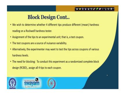
So, this is my example of a blocking for hardness testing, now as I mentioned we was we wish to determine whether 4 different tips produce different mean hardness reading on a Rockwell hardness tester. So, I am using different tips if you have manufacturing knowledge, now whether this tips will produce the same hardness reading or there is a difference.
