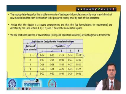
So, this is what I would say that I have 1 nuisance factor operator and I have another nuisance factor batches of raw material and what you can see that each particular operator can only make 5 say particular formulation and you have only adequate amount of say batch of raw material which can prepare only 5 say preparations or mixtures, now in this case I want to simultaneously analyze 2 nuisance factor; one is operator other is batches of raw material.
