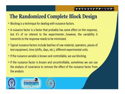
So, what is randomized complete block design? So, blocking as I mentioned is a technique for dealing with the nuisance factor and you may have raw material you have operator shift to shift variation time test equipment as the blocking as the factors to be block and the nuisance variable is known and controllable.
