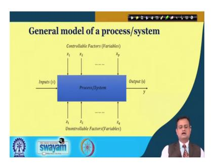
So, you need to have little bit knowledge of this manufacturing process. If you have then you can at least appreciate the input and output of this particular process which is injection moulding. So, we have the input and output and we have controllable and uncontrollable factors. And I would like to minimise the impact of uncontrollable factors. And I would like to set my controllable factors at the optimal level; so, that my inputs can be best converted into the desired outputs.
