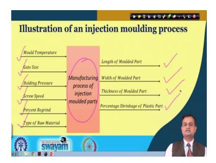
Now, I am just giving you another example that those who are in the manufacturing domain. So, manufacturing process of injection moulded parts, you have mould temperature gate size holding pressure screw speed percent regrind type of raw material as the inputs. And as an output you will have length of the mould part, width of the moulded part thickness of the moulded part and percentage shrinkage of the plastic part.
