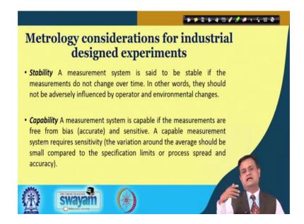
Stability over a period of time if I take the reading my instrument must remain stable measurement must remain stable. Suppose I have checked 1 reading in the morning with Vernier caliper and same reading if I check in the evening that should not be significant difference. In capability so your system is capable if the measurements are free from bias.
