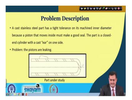
So, let us see, I have the component like this. This is my piston and it is a casted standard steel component and machine inner diameter because a piston that moves inside must make a good seal. The part is closed end and cylinder with cast here on the say one side. So, this is the cast here on this side.
