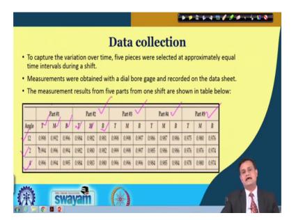
So, you can very well see that I have part 1, and for top middle and bottom I have taken the reading. I have part 2, top middle and bottom part 3, part 4 and part 5. And I have considered the inner eccentricity a 12, 2 and 4 o clock angle.
