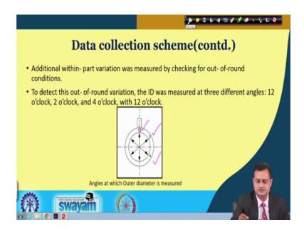
So, I am taking the cross section and this is what you can see that to detect out of round variation, the ID was measured at three different angles, 12 degree. You can see a 12 degree, then 2 o' clock or 4 o' clock. And I am trying to consider this also as a part of my data collection.
