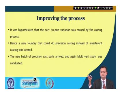
So, this is what I did and typically say you need to improve the process. So, it was hypothesized that part to part variation was caused by causing the because of casting
