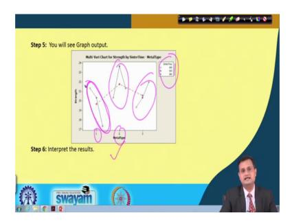
So, you will have another window and your multi-vari chart is available. So, what you can see here again, that this is your sintered time. So, this is for a particular metal type, three sintered time with respect to strength for a metal 2 3 sintered time and this. And you can easily make the inferences that for metal 2, one observation you can make that for metal 2, average strength is higher than the metal one and metal two.
