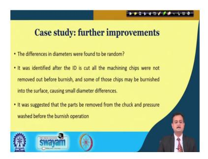
So, difference in diameter where found to be random. It was then unidentified the IDs cut all the machining chips were not removed out of before burnish and some of those chips may be burnished into the surface causing small differences. And it was suggested that the parts we removed from the chuck and pressure washed before the burnishing operation. So, if you have little knowledge on manufacturing, you can appreciate this.
