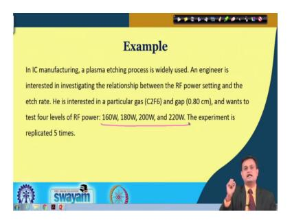
So, this is the first thing that I can check, now I have one way ANOVA analysis in Minitab and you have let us say the data set like this your manufacturing the integrated circuits. And there is a plasma etching process engineer is interested in investigating the relationship between RF power setting in the each rate and interested in a particular gas C2F 0.08 and wants to test four level of RF power 160 180 200 and 220. So, experiment is replicated five times.
