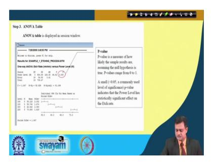
So, basically you get first thing that whether your claim is 2 or not so p is 0.00. So, this is less than 0.05. So, this says that I am in the rejection region, I reject the null hypothesis. So, etching rate for different power setting is not equal that is a difference.
