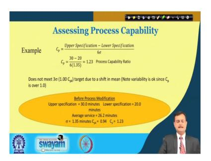
So, this is my process capability index. I would also like to find the C p which basically measures the spread and variability of the process. So, USL minus LSL divided by 6 sigma and I get 1.23. So, here I can say that does not meet 3 sigma which is typically 1 C pk target due to shift in mean. And if we note here, then variability part is C p is ok it is greater than 1, but my C pk has a problem and typically my C pk value is my C pk value here is 0.94.
