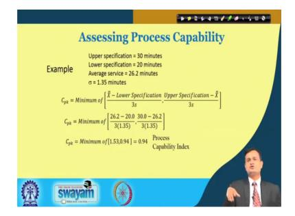
So, I will just plug in the values into my expression for C pk and it basically tags the minimum of X double bar minus lower specification divided by 3s and upper specification minus X double bar divided by 3s. So, computing this I get C pk minimum of 1.53 and 0. 94. So, I will check 0.94.
