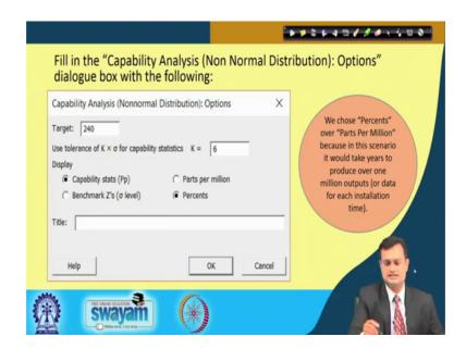
And now with this you conduct basically the process capability analysis. So, you put the target value, you put the k value, that is your tolerance came to sigma. So, six sigma let us say capability stats Pp percent and you try to find out the various values.
