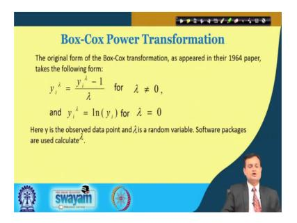
So, Box Cox transformation, the critical element here is the lambda which raises the power of the data to that exchange where your data becomes more normal. So, just see the expression that y i rise to lambda is equal to y i rise to lambda minus 1 divided by lambda for lambda not equal to 0.
