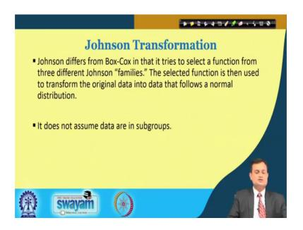
So, you have Johnson's transformation typically differs from Box Cox and the difference is that it tries to select the function from three different Johnson families. SB SU SL and the selected function is then used to transform the original data in case of Box Cox that transformation component was lambda, here you have three distribution families and typically it does not assume the data in subgroups.
