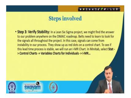
Now, step 3 verify the stability. So, typically in lean six sigma project which we are trying to study for installation of the software, I have a data set, but I would like to check the stability through individual moving average chart and this will tell me that over a period of time my processes in the statistical control or not. If not then there is no point in conducting the process capability analysis whether normal or not normal for the collected data.
