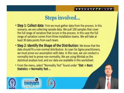
So, steps are very simple to follow, you collect the data identify the shape of the distribution. So, for that step 2 you go to stat basic statistics normality test.
