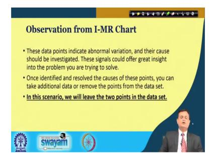
Now I have the observation that these data points which are indicated outside the upper control limit, they indicate the abnormal variation and once identified resolve the cause of this points as I said take the corrective action. And, you can take the additional data or remove the data points from the data set and then you can conduct the process capability analysis for the remaining data.
