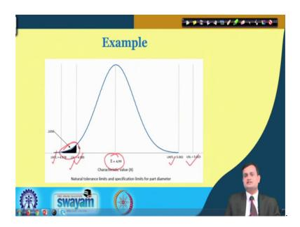
Now, just see here it is interesting, I have upper specification limit 5.015, I have lower specification limit 4.985, I have upper natural tolerance limit 5.002 and lower natural tolerance limit 4.978.
