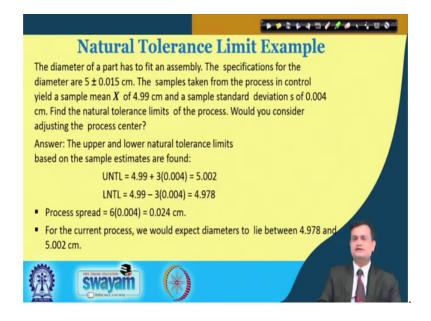
So, natural tolerance limit you can appreciate better through this example that let us say the diameter of a part has to fit and assembly and the specification for the diameter are 5 plus or minus 0.015 samples are taken from the process in control yield a sample mean X of 4.99 and a sample standard deviation of 0.004.
