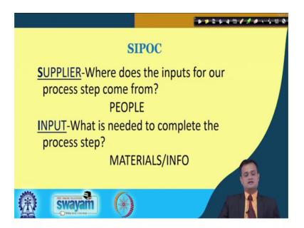
Supplier- where does the input for our process step come from? They are the people supplier. Input- what is the needed to what is being needed to complete the process step? And that is your materials and information.
