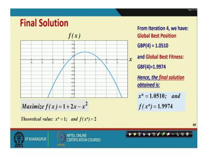
So, this is how the summary that this is the function for which we are trying to find out the final solution Maximize f x 1 plus 2 x minus x square, theoretical value is 1. So, this is 1, x 1, and the value is 2. But what we got through our iteration? We got 1.0510, and f x star is 1.9974.
