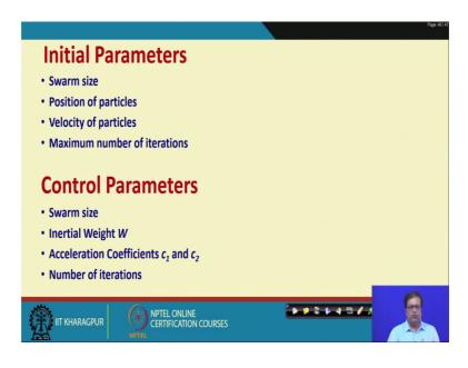
So, some of the initial parameters swarm size, position of particle, velocity of particle, maximum number of iterations and control parameters, swarm size, inertial weight, acceleration coefficients c 1 and c 2, and the number of iterations all right.
