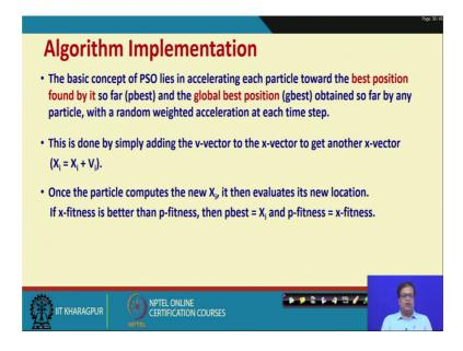
Now, the basic concept of PSO lies in accelerating each particles towards the best position found by it so far that is pbest and the global best position obtained so far by any particle with random weighted acceleration at each state right. And this is done by simply adding the v-vector and x-vector to get another x-vector right. Once the particle computes the new X i it is then evaluates the new location and the p best and the g best and p-fitness and all that.
