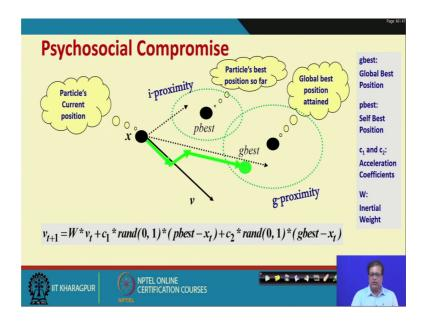
So, I think an example will be very clear for you. So, look here this is an interesting diagram. So, this is the particles current position. So, see look here. So, this is the particles current position. So, one particles current position is this. Now, this is the best possible obtained so far and this is the global best solution obtained so far.
