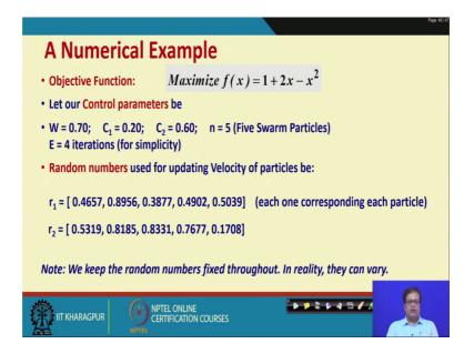
So, let us now look at a numerical example. So, this numerical example is like this. So, first of all objective function is maximized f x equal to 1 plus 2 x minus x square. So, it is a simple problem that we have to maximize these function for the value of x and try to
