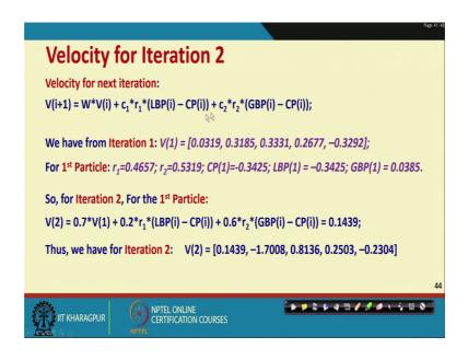
Now, we apply what is known as the velocity that is psychosocial criteria. So, as I have told before, the new velocity will have weight to the previous velocity the current velocity then the c 1 and c 2 two coefficients along with two random numbers r 1 and r 2, the local best position minus current position and global best position minus current position. So, these weight has to be obtained.
