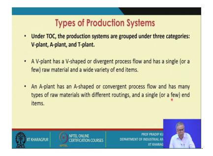
So, as already pointed out let me repeat it once again, under TOC the production systems have grouped under 3 categories ok; V-plant, A-plant, and T-plant. This term we have been using plant ok not explicitly we are saying the V-production system, we have been using V-plant because as we have already pointed out that say your the TOC approach is to be applied at the plant level. And so, that is why you know we have been using this term otherwise it does not have any other significance.
