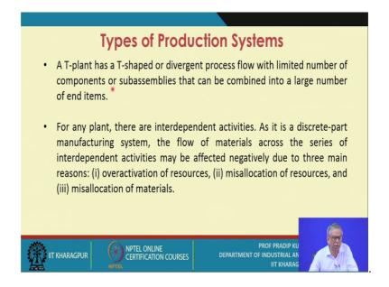
Similarly, you may have a T-plant and this plant has a T-shaped divergent process flow with limited number of components or subassemblies that can be combined into a large number of end items.
