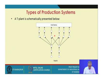
Next you go to the third variety the third type of production system this is referred to as the T-plant. So, a T-plant is schematically presented like this one; that means, you have few inputs you these inputs are further processed, you reach at this stage and then what you do; that means, the multiple say the components of the subassembly you form or you produce multiple components only.
