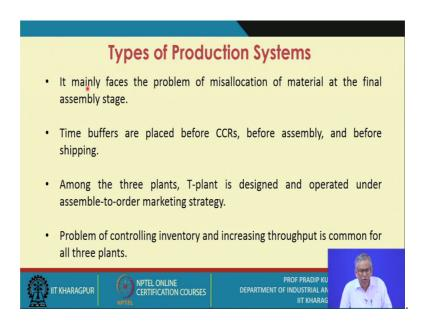
Now, what are the problems it may face? The main the problem it faces that is the misallocation of material at the final assembly stage is it ok; that means the you try to have one particular end item. And, it needs a set of particular parts and a set of particular
