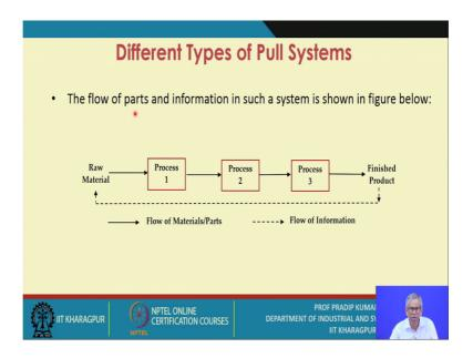
That means the flow of parts and information in such a system is shown is like this; that means, you have process 1, process 2, process 3 and then you have the finished product. And your start in say the system is the raw materials input section.
