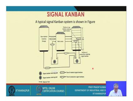
Now, let us talk about the signal Kanban system. Now, as I have already pointed out that in the original the 2 card the Kanban system. What we are assuming we are assuming that the setup time is negligible yes. There are many the manufacturing processes where you know the substantial reduction in the setup time is possible. And so, before you implement the JIT base systems to certain preconditions you have to fulfill.
