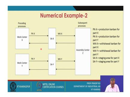
So, this is your the system; that means, you have the work center for manufacturing a part X, your work center Y for manufacturing part Y. And what is PK-X this is the production Kanban for the X item. And this is the production Kanban for the Y item. So now, this is the stacking area. So, the production Kanban moves to the stacking area with the container.
