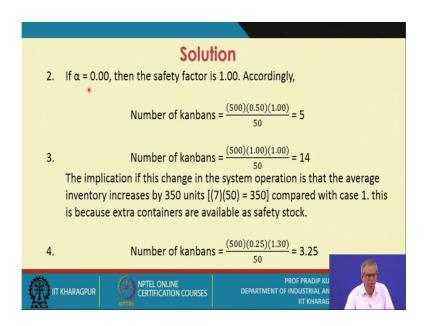
Next is if alpha equals to 0; that means, there is no impact of the external factor. And that is why it is an 100 percent the stable system. So, the safety factor is becomes one accordingly the number of kabanas is 500 into 0.5 into one divided by 50. So, it is reduced to 5, and in the third the case the number of kabanas is 500 that is the daily demand. And this the lead time becomes one day.
