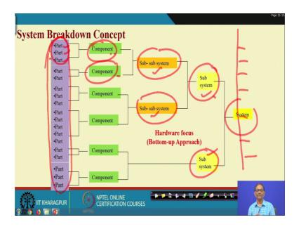
So this is what is our hardware approach, that is bottom up approach. You see what happen a system can have subsystem then can have subsystem then in this sub subsystems con different components and finally, parts. So, we are interested in failure modes here you consider part one part, two part, three like this every part.
