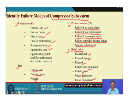
I am just showing you for one subsystem which is basically compressor subsystem. And you have already seen that in compressor subsystem what are the component one is compressor, pipe, pressure control, relief valve. Now, FMEA is also a team game, so your team will have design knowledge, system knowledge, hazard knowledge and obviously, experience that also counts. So, what happened you if you have design knowledge and a hazard knowledge all those knowledge.
