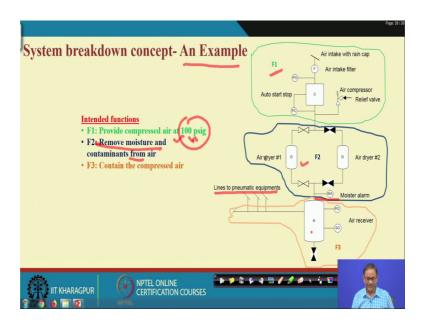
Then you see that: what is the approach with reference to that hardware approach an example. The example is here we are talking about an example is it is a compressor air system. What is actually here is the receiver actually I can say this similar to the pressure tank, that what happened it stores the compressed air and this compressed air is used by line of pneumatic equipment.
