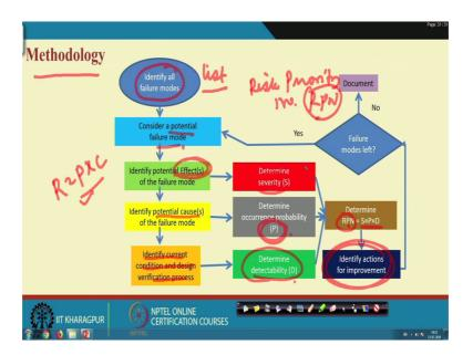
So, once you have failure modes then what is the state the methodology means doing failure mode and effect analysis. What is the methodology? Identify all failure modes, like if you are interested to develop the do go for failure mode and effect analysis of the compressor subsystem, then there are four components and for every component all failure modes are identified, so a list is available.
