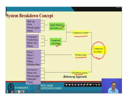
So, now what happen if I go by the hardware approach bottom up approach my totality is compressed air system. You see that compressor subsystem, drying subsystem, distribution subsystem, three things. Air coming to the compressor compress to required pressure then coming the dryer it is dried, then going to the distribution system in the receiver and going to the pneumatic, pnumatic machines
