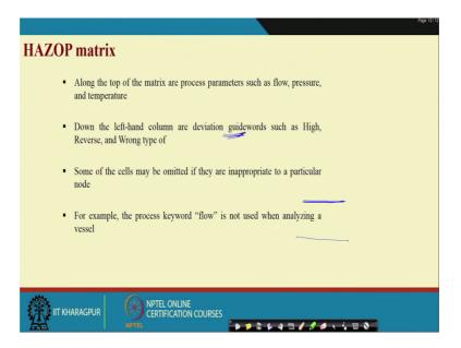
So, then with this background, now you are in a position to develop hazard matrix, and what is this hazard matrix along the top of the matrix process parameters, down the left hand column or deviation of guidewords. Some of the cells may be omitted for example; the process keyword flow is not used when analyzing a vessel let us see what is this.
