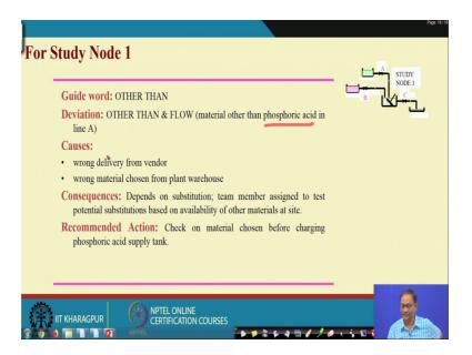
Next other than what is in design intention supply of supply of sulfuric acid. So, you are supplying other than sulfuric acid sorry other than phosphoric acid I am sorry. It is phosphoric acid other than phosphoric acid now phosphoric acid why other than flow means material other than phosphoric acid in line probably varied in sulfuric acid let it be like this then wrong delivery from vendor wrong material chosen. So, these are the causes and consequences you have to find out.
