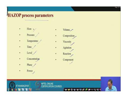
So, common a common process parameters flow, pressure, temperature, time, level, concentration, phase, power, volume, composition, viscosity, agitation, reaction, component, so all may not be applicable.
