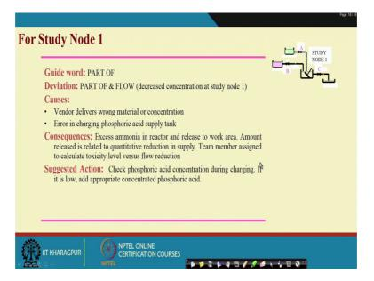
So, this is the way you have to conduct, and then study none 1 flow your writing part of flow concentration is less. Then what are the causes vendor delivers wrong material or concentration error in charging phosphoric acid supply tank, there will be consequences there will be suggested actions.
