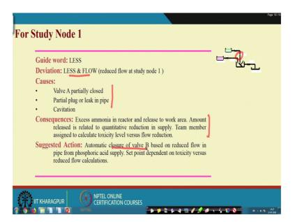
Now, see there may be less flow less flow, so I mean flow is the parameter first one is no flow second one is less flow find out the causes. Find out the consequences you suggest action again automatic closure of valve B.
