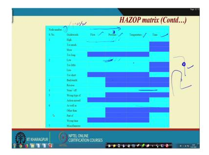
See these are the guidewords these are the parameters sorry this is; what is the parameter, flow, pressure, temperature, time these are the guidewords maybe study node, study node 1, pressure tank. Then what e what guide parameter is important this parameter is important. What will be the guideword high pressure this is or high or more that is giving you the same, similarly too long is not applicable.
