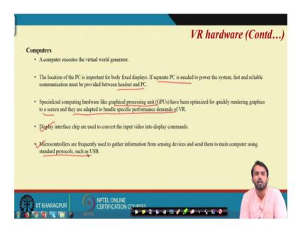
Finally, the computers which executes the virtual which executes the virtual world generation the location of PCs are very much important for body fixed displays. If separate PC is needed to power the system fast reliable and fast reliable communication must be provided between the headset and PC; that means, the connection between the headset, head mounted display and the computer should be that much fast and reliable.
