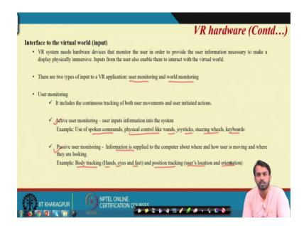
Next the interface to the virtual world; so, VR system needs hardware devices that monitor the user in order to provide the user information necessary to make a display physically immersive. And inputs from the user are also enable to or enable them to interact with the virtual world. So, there are 2 types of input to a VR application that is user monitoring and world monitoring.
