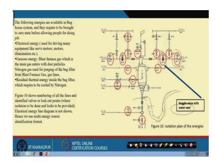
How it is done? First people have to isolate the electrical energies; there are powers all the valves are valves are operated with the power. So, those valves electrical energy also to be stopped; gasses energy also to be at seen and residual thermal energy also to be made 0. That means, once the blast furnace gas line this is the blast furnace gas line, this is better fly valve, this is the butter fly valve.
