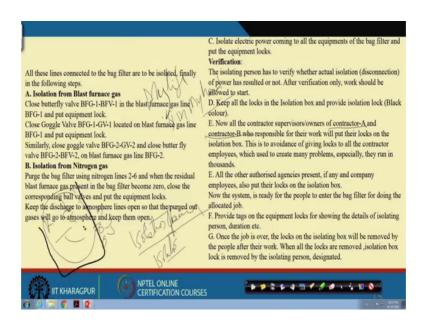
So, I written the sequence. How the valves are to be closed? Blast the lines have been given, names blast furnace gas line, blast furnace gas line one this valve you have to close blast furnace gas line goggle valve you have to close. Blast furnace gas line you have to close this then how to do the nitrogen line nitrogen closing? Then you have isolate the electric power, then you have to verify how do you do verification? By checking inside with a gas meters whether the gas is coming or not?
