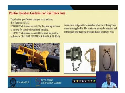
Railway tracks industries railway tracks are there. If somebody is working there people put the flags there not the energy isolation, they put the derailer, this is the derailer. When the when the any equipment comes it will come here and it will come get derailed. The equipment the railway engine will get derailed; on the derailer you put the lock.
