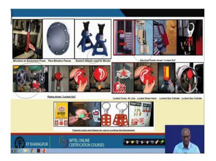
What are the various things we use in these? This is the blank the gas line if you isolate, separate, and put the plan. These are these are the blocks, stoppers for hydraulic cylinder when they lifted. Stoppers when the hydraulic cylinder, you lifted then you put the stock these are the locks.
