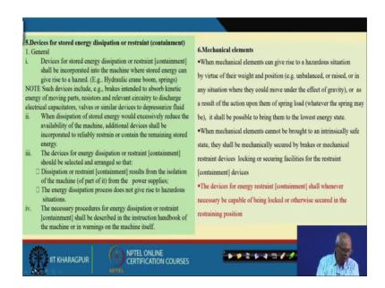
So, the devices which have got stored energy. The devices for the stored energy dissipation shall be incorporated into the machine where stored energy can give raise to hazard. Such devices includes brakes which absorb energy resistors.
