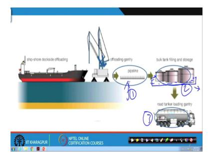
And in this we have identified three hazards scenarios. One is pipeline, other is bulk tankers, third is road tanker. We may select many more sceneries also, but for the case study purpose, we are selected these 3 as the major hazards. Hazards of the pipeline where the where the hazardous material is being carried, hazards in the bulk tank where the hazardous material is stored. These bulk tanks suppose if the any breakdown happens, if it comes out then we have a band.
