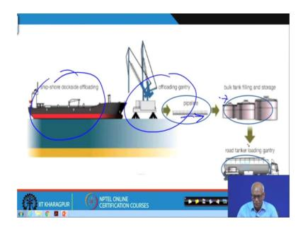
We were discussing the case study. Case study of offshore dockside, where the ships will bring the material, to the off loading gantry, from there it is offloaded through pipeline it will go to bulk tanks, from bulk tank it will go to road tanker. This is a scenario yesterday we have talked.
