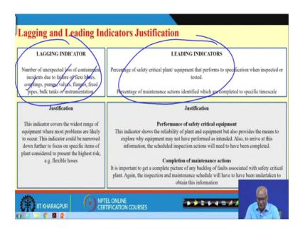
So, lagging indicators, these are the lagging indicators these are the leading indicators, for 1 initiating mechanism it is showing 1 line, but the total data is numerous from here. You should have lagging indicator of data of flexible hoses, couplings, pumps, valves, flanges all these things. It becomes big data.
