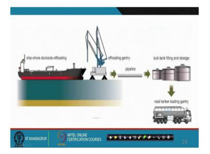
This is this is the offshore a ship coming and unloading the various materials into the offloading gantry through the offloading gantry, through the pipeline to the bulk tank filling and storages. From there it will be loaded into road tankers, it will be dispatched to the customers. This is the case study we are taking.
