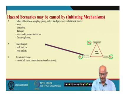
What are the initiating mechanisms? Failure of flexible hoses, couplings, pumps. The failure of flexible hose pumps valve fixed pipe, why do they fail? Because of the because
