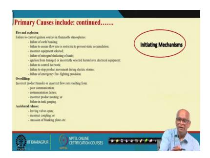
What are the initiating mechanism for fire and fire and explosion? Failure of earth bonding, failure to ensure flow rate, incorrect equipment selection, failure of nitrogen blanketing of tanks, or failure of control hot work you are not controlled properly. Hot work hot work means welding and all these things. So, a spark as come and has fallen a some cloud. So, whatever initiating mechanism for overfilling poor communication people are not communicated, so overfilling.
