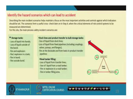
What are the hazardous scenarios here? Hazardous scenarios means in our in our safety triangle we called hazardous elements. In the whole process which we are discuss storage tanks is one of the hazardous element. So, what will what will happen in the storage tanks? Loss of liquids loss of liquids in the bunds, the liquid the tanks will have bund. Bund is if any case if the any leakage happens the bunds will hold the liquid it will not go to outside.
