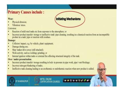
Some more initiating mechanisms physical abrasions, vibration corrosion; so, corrosion by the corrosion will happen, corrosion will happen because of the reaction of the milds with the mild steel.
