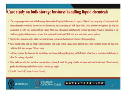
So, case study shows the company operates constant bulk storage business handling, chemicals. So, there is an offshore at the offshore there are a tankers provided it is they are called bulk tanks. They are all loaded into the bulk tanks through the pipelines it
