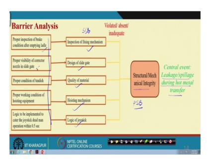
Then we have seen barrier analysis. So, barrier analysis here we are showing you once barrier analysis where leakage and spillage during hot metal transfer. So, it can be because of structural mechanical integrity, because of operator's integrity, because of many other reasons.
