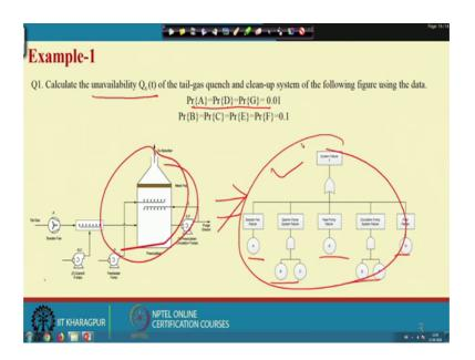
The question is calculate the unavailability of the tail gas quench and clean up system, this system you have already seen, this is the tail gas quench system and the fault tree of this tail gas quench system is given. Now we have to find the unavailability, the basic event probability is given here, the probability of A, probability of D all the things are given here. So, I will show the step by step procedure that, how to calculate unavailability given this fault tree.
