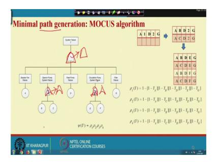
So now, we will go for minimal cut. So, you have seen the minimal path. Now, I will go for minimal path. So, in minimal path for calculating the minimal path set there are again 2 option, first option is you have to just convert OR gate in to AND gate and AND gate into OR gate and then you just take the same way that, you have done in minimal cut representation means, you have to find out the minimal cut of this conversion fault tree.
