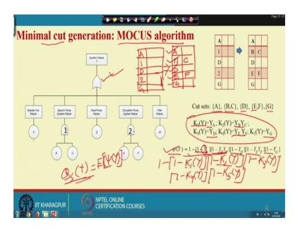
So, you can see that this is my fault tree. So, for getting the minimal cut of this fault tree, we have to use the MOCUS algorithm. So, what is MOCUS algorithm? Suppose this is my matrix, 2 3 ok. So, the input to this OR gate, are A then 1, then D then, 2 then G. So,
