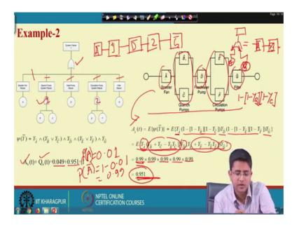
So, you can see that how to form the reliability block diagram from the fault tree. So, look it is OR gate as it is OR gate and this, the inputs are A then this AND gate suppose this AND gate is 1, I have naming it then, this is C, this is 2 then this is G. So, these are the input. So, as this is OR gate, we can write the RBD, this will be A bar in series, it will be 1 as the from the property of OR gate, we know that if this is OR gate and this is A
