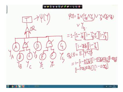
So, first I will draw the fault tree, suppose this is my top event then, there is one AND gate sorry OR gate, this is OR gate, now the basic event A then input is AND gate and the basic events are B and C. Now this is another basic event D, again another AND gate inputs are E and F another basic event that is G.
