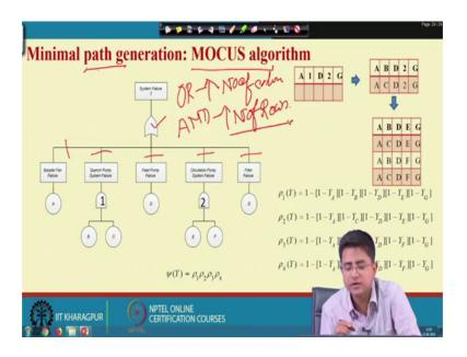
So, when you will put here AND gate suppose, there is 1 AND gate and now OR gate and you take the minimal cut representation of this fault tree, convert converted fault tree, then you will get the minimal path, but I will show another the same MOCUS algorithm, during minimal path generation. So, we will not convert our fault tree, it will
