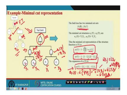
Let us concentrate on this example. So, this example, this example, this is the fault tree, A B C basic events, 3 basic events, it is an and gate, this is OR gate, this is the starting point. We have converted these 2 equivalent fault tree using cut set of this fault tree. What are the cut set, cut set will be what will be there will be 2 cut sets, A must occur, B or C occurrence will lead to so, A B and A C. So, there are 2 minimal cut sets A B and A C.
