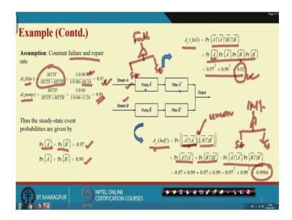
So, the first one, what is the assumption here that we are assuming that constant and failure and repair rate for both pump and filters. So, if this is the case then, you have seen earlier when we have discussed quantification of basic events that time we have shown you that availability is A can be measured by mean time to failure divided by mean time to failure and mean time to repair. This means with this equation availability is measure.
