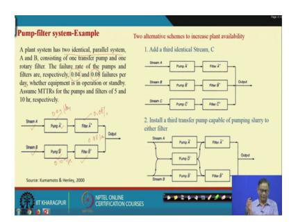
Now, we will see one interesting example here, this example we have taken from the book Kumamoto and Henley. Here the issue is, I am just reading out the description of the plant, plant has 2 identical parallel systems, so known as stream A and stream B. So, stream A and stream B they are identical, but parallel system. So, both the stream consists of 1 pump and 1 filter in series and two stream are in parallel ok.
