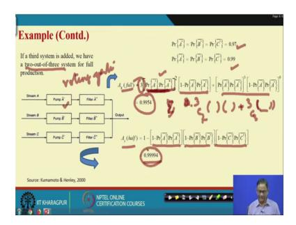
For 3 identical stream A B C, so again the as identical that mean the pump A B and C they are availability or probability of successfully working is 0.97 and then the ok, A B C 0.99 and 0.97. So, A star, B star, C star that is basically the filter and A dot A dot B dot C dot or A dot be a double dot B double dot C dot filter, this is simple you know what is already written here ok.
