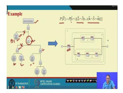
So one example, this is the pressure tank example, several times we have discussed, what is this pressure tank. Our issue is pressure tank rupture and considering only the primary failures or the basic events and ignoring the your secondary events, the poultry is simplified to this part, this kind of poultry.
