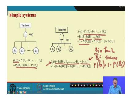
Simple system, simple system means, the system can be represented using AND or OR gate or maybe and our combinations ok. So, if the top event is linked with the bottom basic events, with AND gate you all know what is the probability of the top event occurrence, if top event occur at time t, then it is basically system is unavailable.
