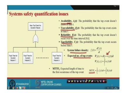
Now, let us spend some time here, that what are the issues that is important for system safety quantification. So, if you recall the fault tree and finally, the cut sets for fault tree or different kinds of hazards, that alone or in combination with different events lead to the top event.
