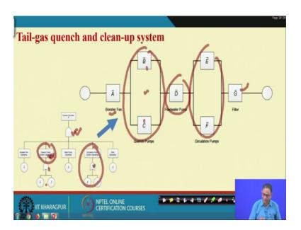
Now, this one can be equivalently represented by reliability block diagram ok. So, that is what is written here a booster fan, there is or gate parallel system, then and this one is basically with AND gate, in the series another or gate parallel this is with AND gates series.
