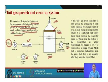
So, I I hope that we have given enough explanation to RBD and then fault, fault tree and RBD linking here, I am just giving another example, which we have taken from the Kumamoto book. This is a system, where basically some hot tail gas is coming from calciner and it is basically through booster pen, it is coming to this quenching system.
