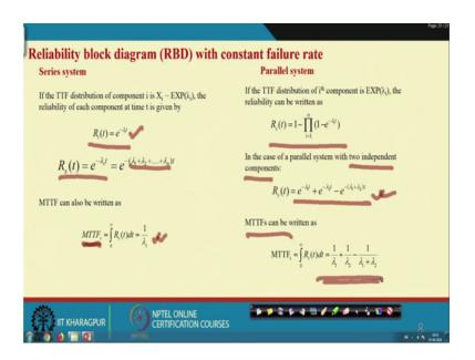
So, let us see some more related to this. Now, what will happen, if the components are having constant failure rate? So; that means, the time to failure is exponentially distributed under this situation, what will be the reliability? Reliability will be for component, reliability will be this, where lambda i is the distribution parameter exponential that distribution parameter for the ith component.
