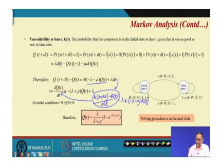
So this can be written this can be written as Q t plus delta t minus Q t by d t equal to this much so, lambda plus minus lambda minus mu Q t. So, now, this quantity is nothing, but del Q t by d t that is what is written here.
