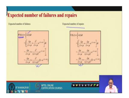
So, you can calculate expected number of failures once you have unavailability you are getting w t. So, once you have small w t, then that expected number of failure ok. This is 0 to t time you just integrate w t d t 0 to t this integration will give you this equation. And expected number of repair will give you this equation.
