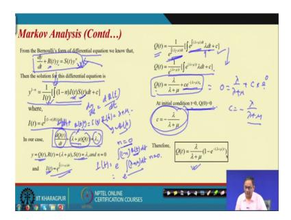
This is the equation Bernoulli form of differential equation. First order del y by del t R t y, S t y to the power n. If your differential equation of this form, then the solution to this equation will be of this form. Where I t is this e to the power integration 1 minus n R t d t.
