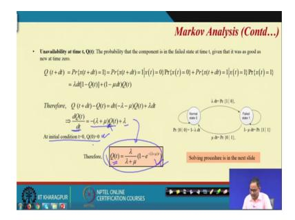
So, del Q t by d t equal to this plus this; this is the first order differential equation. So, you have to solve this equation and if once you solve this we will see the one only formula. That once you solve this given this condition t equal to 0 unavailability is 0 the solution to this to this differential equation will be this; Q t equal to lambda by lambda plus mu 1 minus e to the power minus lambda plus mu into t.
