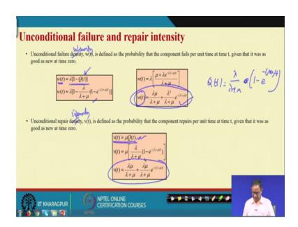
So, if you know unavailability equation and we have seen in the last class that the how this unavailability is related with unconditional failure intensity and unconditional repair intensity, last class you recall. So, we have written there the w t is unconditional failure intensity which is lambda into availability.
