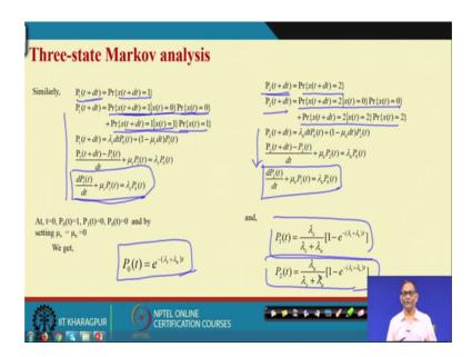
So, in the same analogy the way we have found out P 0, t plus delta t you have, you will be able to find out P 1 t plus delta t. So, p 1 t plus delta t means it is in state 1, then this is nothing, but that it is in the state 0 transition takes place to state 1 into that it was in state 0 plus it was in state 1 remain in state 1. There is nothing related to we have not considered anything related to the transition from fail safe to unfail unsafe or fail unsafe to fail safe.
