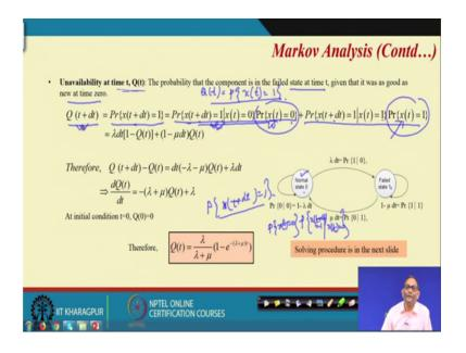
So, you have seen in fact, you know that; what is your unavailability. So, unavailability the probability that the component is in failed state at time t equal to t, given that as it was as good as new when time t equal to 0 ok. So, Q t means what you can write Qt probability x t equal to 1. Now then we can write Q plus delta t equal to probability that x t plus delta t equal to 1.
