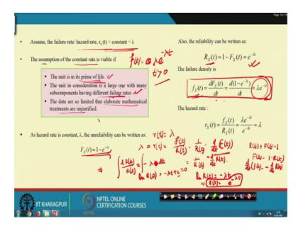
So, if failure rate is constant, that mean  $r \times t$  is lambda, then you will see that from here using this  $r \times t$  you will be able to device all those things. So, I will write down here. So, our  $r \times t$ , I am not writing  $x \times t$  I am only writing  $r \cdot t$  so, this is lambda. Again, you know that  $r \cdot t$  is nothing, but  $f \cdot t$  by capital  $R \cdot t$ .
