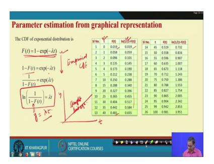
So, it is our, it is one of the another advantage of exponential distribution. Now, suppose a you have data and you want to find out the lambda values graphically. From theory you have seen that the lambda value is 1 by mean time to failure, the reciprocal of mean time to failure or a, but here what happened. Suppose, you have data and you want to find out the, what will be the lambda value (Refer Time: 19:39) from the from plots.
