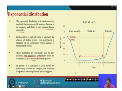
So, I again rely on this hazard rate curve, because the because exponential distribution and the constant failure rate, they have huge relation. Basically, if the hazard rate is constant which is basically the time of useful life. And, then you will see later that the failure distribution density will be exponential distribution.
