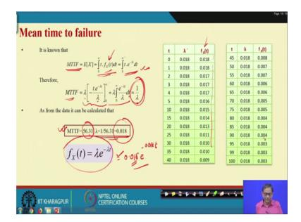
So, now let us see the example is a the is the same what we have discussed in last class last, but one that class also. We have given you some 100 data points and then from that data what we have calculated? We have calculated the mean time to failure mean time to failure.
