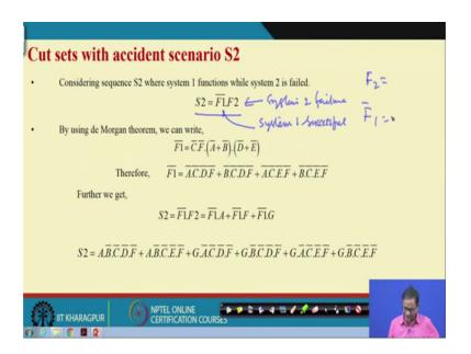
Let us understand for the S 2. So, let us see. So, you all know that what is S 2 when F 1 mean system 1 successful, system 2 failure, ok. Now system 2 failure F 2, what is the cut set and F 1 cut set, if I ok, it is already there, fine.
