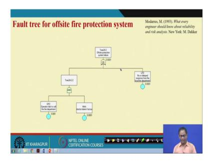
Now, you can find out the offsite on the also that will fail um. So, in a similar manner you find out the fault tree for this event tree for this. So, that mean what i mean to say what I have shown you here not only fault tree here, fault tree here fault tree for this, fault tree for this also because otherwise how do know it is working the pivotal events
