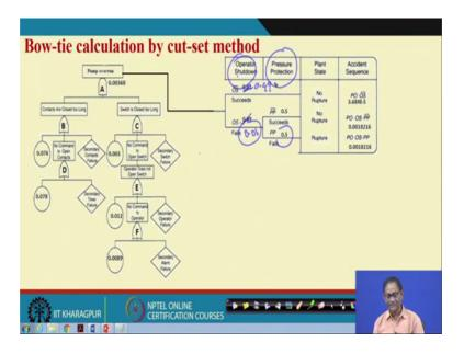
Here what happen we are saying operators shutdown and we are writing that operator shutdown fails with 0.01 and succeeds 0.99 ok. So, now, how do you get this probability? So, that mean there maybe or pressure protection it suppose fails 50 percent
