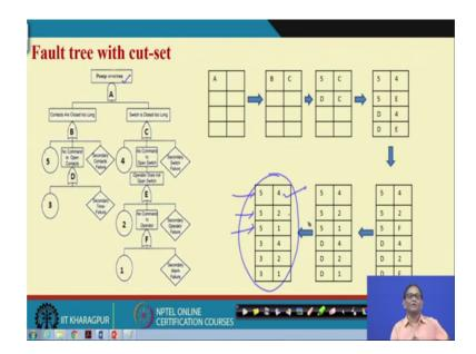
Now, I will just repeat the case the cut sheet case for this. These are the cut-set earlier we have discussed how to develop cut-sets. I am not going into why not going into that detail of cut-sets. So, you say that there are 6 cut-sets two any this occurs this will occur this occur this will occur. So, what will be your preventive measures here you do something. So, that this two simultaneously these two simultaneously, this two simultaneously this should not occur ok.
