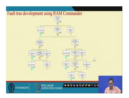
Now, here we are basically we have used RAM commander and we have developed this fault tree. And this fault tree can be manually developed also so that also we have seen. But thing is that we want to see all the that cut sets as well as the importance measures from this because manually computing those importance measures will be difficult in the sense that may not be possible also.
