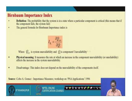
Let us see that what are those measures available, the measure first measure is this Brinbaum importance index. What it is given to us? It given that the probability that the system is in a state where a particular component is critical ok. Suppose the tank our the pressure tank the system, the system will be under normal state under, abnormal state may be over pressure condition or maybe the rupture condition that is tank rupture.
