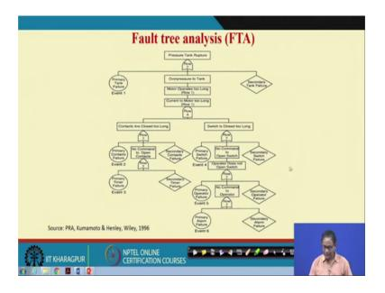
So, you see that is what we have developed here and I have taken these from this book it is already developed there. So, pressure tank rupture this is the system level mishap or accident you do not want this rupture to take place. So, as a result you want to know; what are the reasons of pressure tank rupture and what are the basic events that alone or in combination contributing to the pressure tank rupture?
