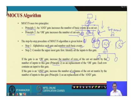
Please listen very carefully that how mix MOCUS algorithm works. So, it is very important algorithm for fault tree analysis. There are 2 principles. Principal 1 and principal 2, it is basically related to AND and OR gate. So, when you develop a fault
