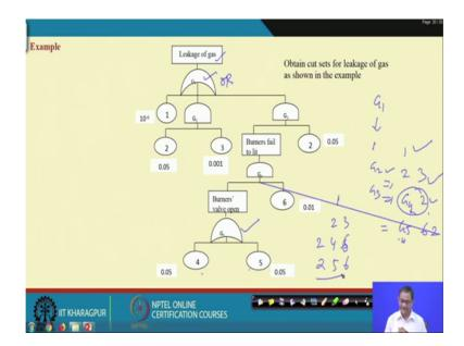
See the situation here leakage of gas OR gate, how many inputs? 1, 2, 3 so, if you want to create so, first you start with G 1, then it is OR gate, it will increase the number of rows 1, G 2, G 3. So, these are all cut sets.
