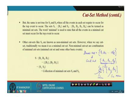
For example, B 1 B 2 to B 6, then we say cut set. For example, B 1, B 2, B 3 this is a cut set. Why it is cut set? Because this 3 basic event if occur, the top event will occur. It is not basic set because basic set contents all the bottom level events.
