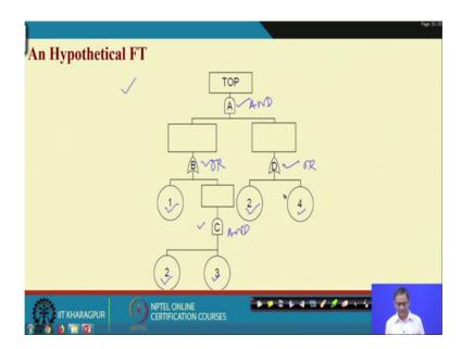
Suppose this is our hypothetical fault tree. Top event alphabetised gate A, gate B, gate C gate D. This is my AND gate, this is another AND gate, then this is OR gate, this is OR gate. Now number the basic events 1, 2, 3, again 2, 4; that means, this events coming in the 2 places of the fault tree.
