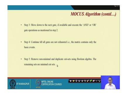
And then what happened? You move down to the next gate. And in this process go down to the to the bottom, bottom level and then you will having lot of cut sets. And then all non-minimal and duplicates cut sets will be will be removed using Boolean algebra, then the remaining cut sets will be the minimal cut sets.
