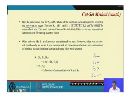
So, now what we have found out? We found out that the from the arbitrary sub selection of subset like S 1, S 2, S 3 and S 4 this is cut set, cut set, not cut set, this is cut set,. So, what happen in S 1 and S 4? All the events in the set required to occur for the top event to occur let me go back again.
