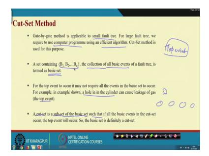
So, you have already seen the gate by gate method in gate by gate method, the top event with different gates finally at the bottom events. The bottom event probabilities is known, and every gates are quantified and finally, top event probability is quantified. So, that method is good for small fault tree. For large fault tree, you required to use computer programming and you require an efficient algorithm for that purpose.
