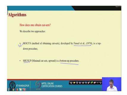
So, how do you generate cut set? We will use MOCUS algorithm developed by Fussel et al 1974. It is a top down approach or mix up; that is minimal cut set upward it is a bottom up approach. Both the approach are more or less similar. So, but one is from top to bottom another from bottom to top so, we will discuss this approach.
