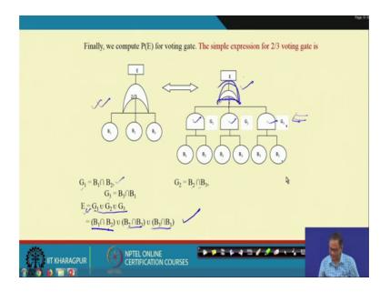
So, what we are doing here first this voting gate 2 by 3 gate is represented in equivalent or and AND gate this is AND gate or and AND gate. So, if 2 out of 3 occurs top event will occur. So, then if B 1 B 2 occur top event will occur B 2 B 3 occur top event will occur or B 3 B 1 occur top level will occur.
