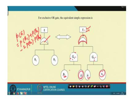
Now exclusive OR gate we are seen that P B 1 p p probability of E what you have seen probability of E P B 1 plus P B 2 minus 2, P B 1 P B 2 what is exclusive OR gate that, either of the 2 one should occur, but not both. So, its equivalent this is exclusive OR gate its equivalent or and representation is this. So, B 1 should occur B 2 should not occur that is why B 2 bar. Here B 2 occur, but B 1 should not occur that is B 1 bar.
