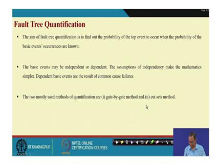
So, let me repeat the aim of fault tree quantification is to find out the probability of the top event to occur when the probability of the basic event occurrences are known. The basic event may be independent or dependent, the assumptions of independency make the mathematics simpler dependent basic events are result of common cause failure.
