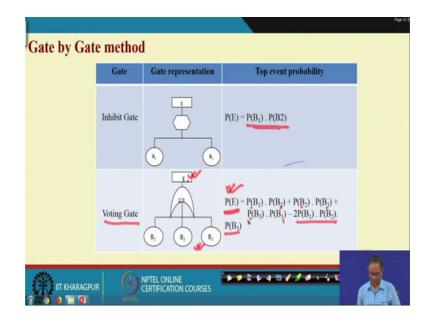
Now the last one from the last 2 inhibit gate and voting gate. So, we have discussed that inhibit gate in the last class and you have seen that it is nothing, but that an AND gate equivalent AND gate. So, that is why what happen in case of inhibit gate the top event will occur only both the event will occur and it is the intersection. Please remember we are basically talking about all the cases independent basic events.
