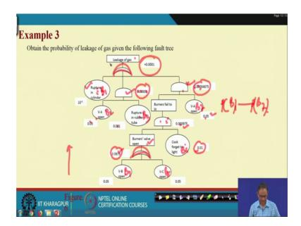
Now leakage of gas case see here. So, these are the basic events suppose this is B 1 this is B 2 then this one is B 3 B 4 B 5 B 6 let it be B 7. So, you have data one B 1 B 2 B 7. So, B 1 to B 7 these probability data that mean P B 1 to P B 7 this data are available with you.
