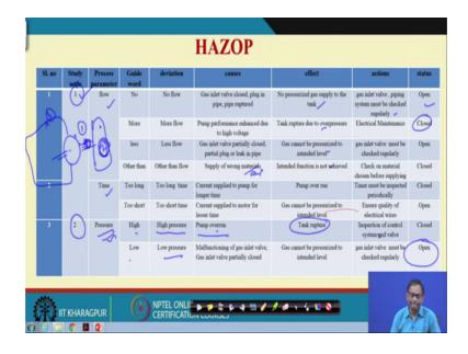
Then HAZOP or HAZOP purpose so, you have to find out the study note we have considered 2 study note, the 1st study note is the wire from pump to pressure that that is the best there is a pipe and there is pump and rest of the things like this so here one study note is taken. So, this is the 1st one and the 2nd one is the so 1 and 2, 2 different study note we have taken.
