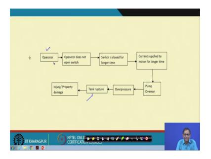
So, in this manner we created the ontology works in path 5, 6, 7, 8 now 9 operator, operator does not open switch; switch is closed for longer, time current supplied to motor for longer, time then pump overrun, pump overrun leads to over pressure, over pressure leads to tank rupture tank rupture lead to injury property damage ok.
