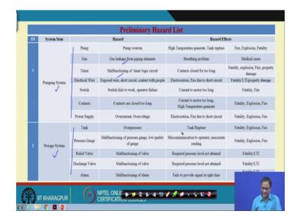
Now, for the same thing we have we have to develop the preliminary hazard list, the pumping system having this many components storage system having this many components for every component the hazard, hazard effects and means basically the hazard initiating mechanism target and threat and these are the hazard elements. So, these things we have written and we have found out several basically hazard this list pump overrun, gas leakage, malfunctioning so like this many things we have created here.
