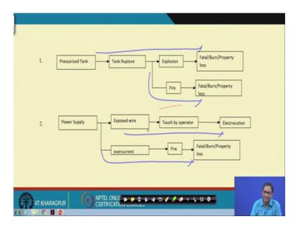
For example pressurized tank, tank rapture, explosion fire, this is one path, this is another, here power supply related one path electrocution, another path related to fatal
