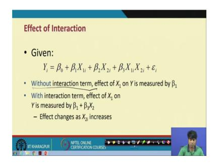
So, here in the same structure so; that means, a the model is the Y equal to beta 0 cross beta 1 X 1s beta 2 X 2 and beta 3 X 1 X 2 where you know we have you know without intercepts interaction term.
