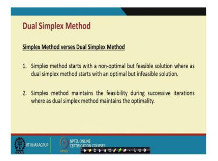
So, let us see here the kind of dual simplex mechanisms. So, simplex mechanism and dual simplex mechanisms; simplex method starts with a non optimal, but feasible solution where as dual simplex method starts with an optimal, but infeasible solution. So; that means, it is just you know counterpart kind of things through which you can address the business problem. And simplex method maintains the feasibility during the successive iterations whereas, dual simplex method a kind of optimality/.
