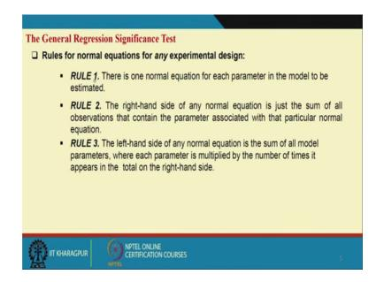
So, this is the rules. Now, for normal equation that there are three rules. Rule one is there is one normal equation for each parameter in the model to be estimated. So, we have in one factor one way ANOVA, we have a levels for a treatments levels and grand mean.
