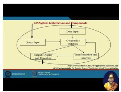
So for tracking the vehicles, tracking the consignments across the supply chain, beyond the coverage of RFID, the systems that are used are GPS-GIS integrated systems. So this GIS system, this is a schematic diagram of GIS whether data input comes from GPS and stored in the geographic database, then it can help in answering the queries of the user and generating reports and it has capability, some capability of transforming and analysis of the data.
