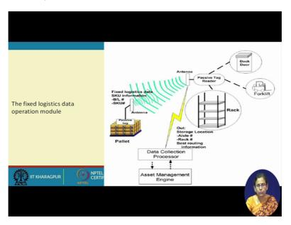
Now the data see we have two types of RFID tags. One is passive RFID tags which is attached with the pallets and stock keeping units and we have active we have some active tags which are attached to the metal handling equipment. So now the antennas collects the passive the this pallets which add items they are in which are attached to the passive tag once they come under to under the field of the passive tag reader they will be emitting the data details.
