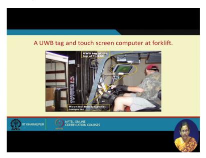
And this is what I was talking about the driver who is moving around the warehouse he will be sitting on this on this matter handling equipment and he has a touch screen computer where the details of the picking sequence will be shown.
