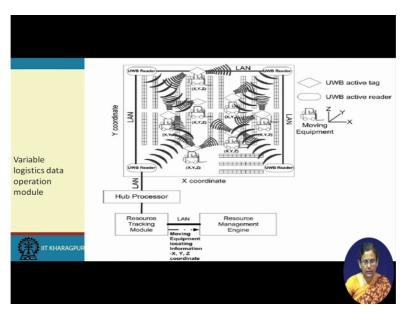
Now this data across this is an example that we will showing and it is also wifi enabled LAN is there and antennas are accordingly positioned. So this signals come from many directions and they are sent to appropriate resource tracking module. Their positions will be their positions and details will be sent to the appropriate resource tracking module.
