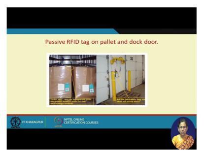
Look this is some examples where the pallets are attached with the RFID tags. Even the RFID in the side of the back door also there is a RFID tags attached.
