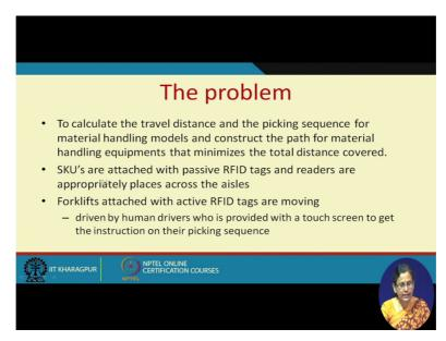
Okay so SKU's are attached with passive RFID tags and readers are appropriately placed across the aisles. Now forklifts attached with active RFID tags. This material equipments with forklifts are they attached with active RFID tags. Now while discussing about RFID we are talking about active RFID. Active RFIDs are basically used for asset tracking.
