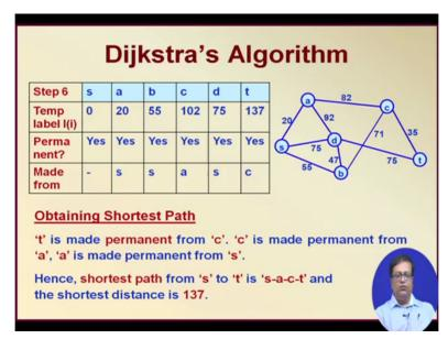
So now this is our complete table. These are the labels no more temporary, they are all permanent. If all the levels are permanent and made from least is also available. So what we do t is made permanent from c, c is made permanent from a, a is made permanent from s. So
