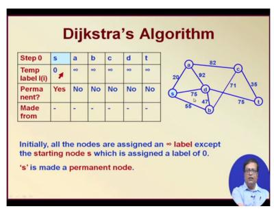
Now after the distance matrix is obtained you see, first we have made s permanent right. s is made permanent and temporary level is assigned to s as 0, then a,b,c,d,t all the remaining nodes they are assigned as infinity as the your temporary level. Now is anything is
