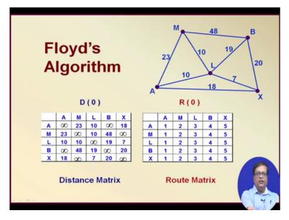
So we make 2 matrixes, the first matrix is call the distance matrix and the second matrix is called the Route matrix. The distance matrix is you know the distances like infinity A to A and you know they are all infinity, X to M there is no such path. So it is also infinity, then like
