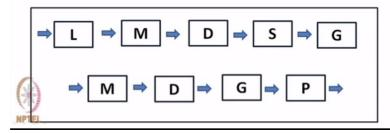
This is an example of product layout, which is in line fashion. The operational sequence and the machine arrangement are the same.
