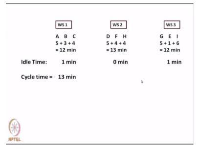
Now what we do here we have transferred G from workstation 2 and H of workstation 3 that means we have brought H here and G we have taken there. So G has gone here with 5 as the element time and H has come here with 4 as element time. Thus, here it is 13 minutes instead of 14 and here it is 12 minutes instead of 1 that is the idle time is to extend of only 1 minute and the total cycle time is 13 minutes.
