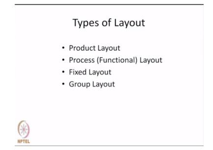
We said that there are principally 4 layout patterns, product layout for product focused systems, process or functional layouts for processed focused systems or (()) (01:52) problems, the custom products, fixed layout for very big and heavy products and then a combination of product and process that manifests itself in the form of group layout.
