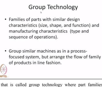
A variation of that is called group technology where part families are made based on similarity of the design characteristics and of manufacturing characteristics. Design characteristics with regard to size, shape and function, manufacturing characteristics with regard to type and sequence of operations. So they are like group layout but there is a difference.
