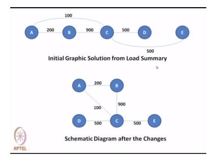
So what is now done is that from these values we construct an initial graphic solution where we show almost in a linear fashion first of all, all the departments or operations. So these are A, B, C, D, E and the quantity traveling between various departments are written down here along the arc that joints these notes. So between A and B the amount traveling is 200, between B and C 900, C and D 500, A and C 100 and C and D 500.
