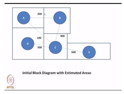
Once this space is estimated for every department, we already know the relative location of A, B, C, D, E. Now this space requirement for A could be this, for B it could be this, for D it could be this, for C it could be this, E it could be this. So first of all we make an initial block diagram with estimated areas. Now you can see that this is very irregularly set but the actual set could be a rectangle or could be a square.
