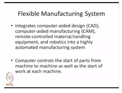
And today we are talking about flexible manufacturing system where computer-aided design, computer-aided manufacturing, remote-controlled material handling equipment and robotics makes the manufacturing system almost fully automated and here the human intervention is much less during manufacturing and very high during the designing and process planning stages.
