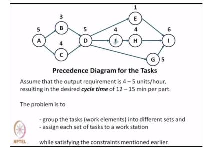
D, F, and H all the three after D is complete F can be completed and after F is complete H can be completed. Earlier D, F, and G were put in one workstation, now what we have done, we have put G to workstation 3 and from workstation 3 we have brought H to workstation 2. So 5, 4, and 4 is 13 minutes is spent in workstation 2 and workstation 3 is busy for 1+6+5=12 minutes. This trade and transfer was done purely based on trial and error method.
