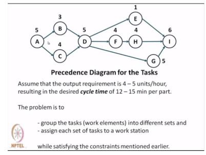
It can be represented in a network form A, B, C, D etc the work elements and the operation times or element times are given in number. So we have to group these operation times and assign them to various workstations such that precedence relationship is not violated, meaning that D cannot start unless both B and C are complete. So basic constraint must be satisfied.
