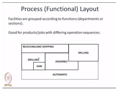
In a process layout, different machines or functions are grouped together in the form of a department and they are placed together.
