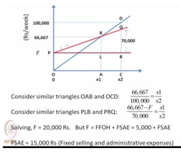
This is the breakeven chart, the revenue, the fixed cost and the total cost. Now here, this is the breakeven point and this is the actual value at which the company is operating and it has made some profit. Now, if we consider the triangle OAB and triangle OCD they are similar triangles. Therefore, we can now look at this it says the breakeven sales is given as 66,667 whereas the actual sales is 100,000.
