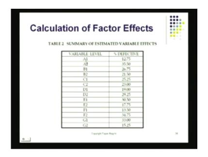
Now, this is the data that was then analyzed and how was this done, we calculated the averages and I am going to show you one or two examples of this calculations. I am going to be just taking a little sheet of paper here. And I will use my calculator I am going to be working out for example, for A 1 we are going to be finding this percent defective, let us do that.
