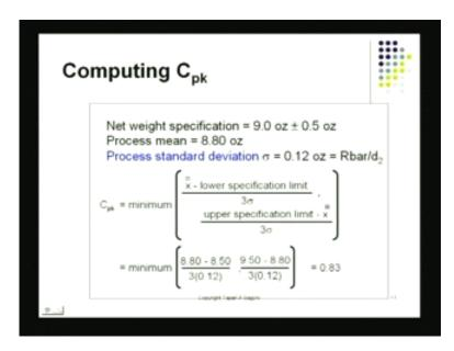
And if I show you calculation here is a little calculation I use the same data that we had before my tolerances were given as 9.0 plus or minus 0.5 ounce process mean this the x double bar turned out to be 8.80 by actual measurement process standard deviation turns out to be sigma which is 0.12 ounces and this I formed by calculating R bar by d 2. Remember this; what we also used in one of the earlier calculation when we were doing s p c.
