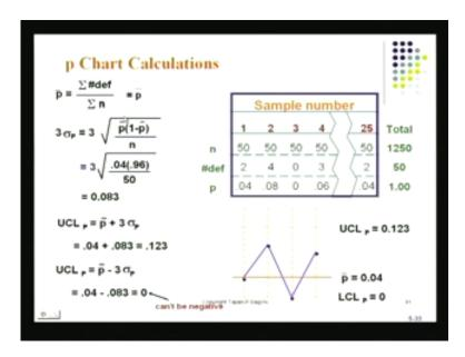
And those are done here, look here, the p bar turns out to be this and I use my control limit calculation, I find my sigma p, three sigma p then and I find my upper control limit which is 0.123 and lower control limit turns out to be 0, because it turn out to be negative, so I made it 0. And then, I low and behold, I got the neural control chart there, everything is in control, because the upper control limit is way out there so on.
