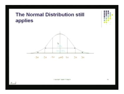
So, in fact we are still using the normal distribution as our, to try to locate the points that are like the extreme situations, when the process is under under normal control, under statistical control and that we do just by again plotting the plotting the chart in such a way that, we got these upper and lower control limits at three sigma p this times, on the high side and also on the low side, around the average.
