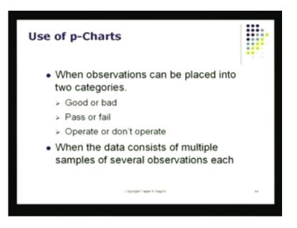
And I will show you the limits for these also. So, in fact what are we talking about, we are talking about quality characteristics that could be measured, not that cannot be measured, but can be just on a good or bad basis, pass or fail basis when data consists of characteristic like this, we would utilize the p chart.
