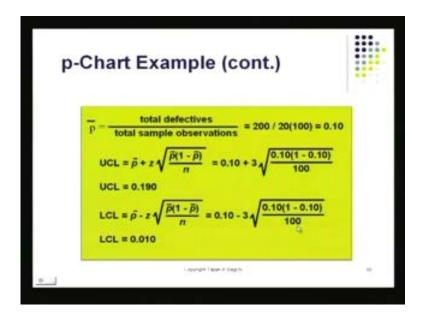
So, for that I just go to the control limit formula and the value of z this time I am going to be taking three sigma limits. So, I put down 3 there and these the value of sigma p and I have got that quantity put down there and if you do the calculation, you will find that the upper limit turns out to be 0.190 and lower limit turns out to the 0.010 which really says, if the value of p if the value of p, p is the fraction defective in any of those lots of size a 100.
