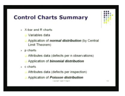
So, again I could construct the c chart there. Now, let us take a look at what sort of things we have been using, for the x bar and r chart, we use the normal distribution to find the control limit, for the p chart we use the binomial distribution as an approximation to normal distribution, it became a approximate into a normal distribution and then, for the c chart, these were counts out defects, we use the Poisson distribution.
