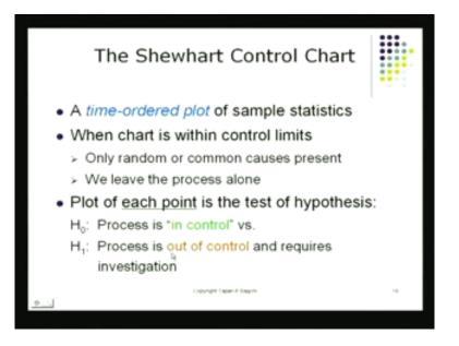
So, what is a control chart? It is a time-ordered plot. That is what this is and it provides you with a signal. When there is no special cause impacting the process nothing has gone wrong, nothing perform has happened to their process and the process remains within what we call your in control is a in control state. And of course, if some wild things happen in the process like a tool breaks down or the raw material is changed or a operator comes along and he starts operating the machine.
