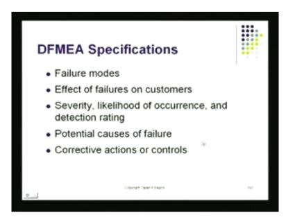
So, that this failure does not really take place, that is something that you would like to do. D F M E A come ups design failure, mode analysis. This is actually comes up with failure modes, the effects of the failures, the severity or the likelihood of the occurrences
